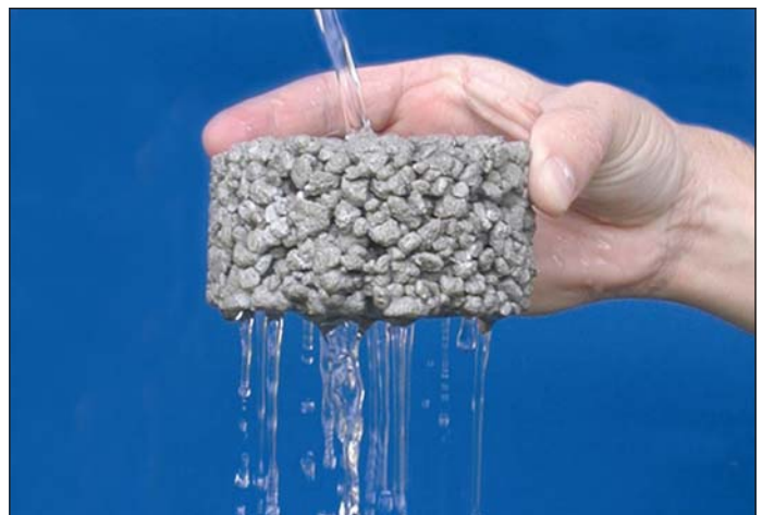
Figure 5. Pervious concrete is used for parking areas, streets, plazas and walkways to help minimize stormwater runoff to surrounding streams and lakes.
